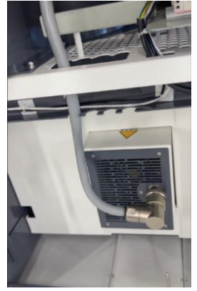
Figure 20. Install Connector on the Emitter Connection Port
