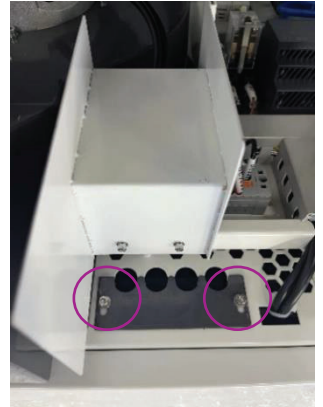
Figure 16. Loosen the Screws; Remove the Wire Pressing Plate
