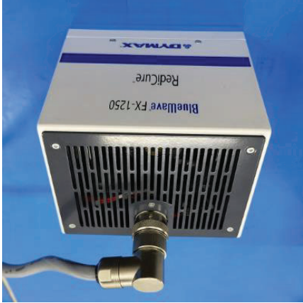
Figure 32. Plugging Connection Cable into Emitter
