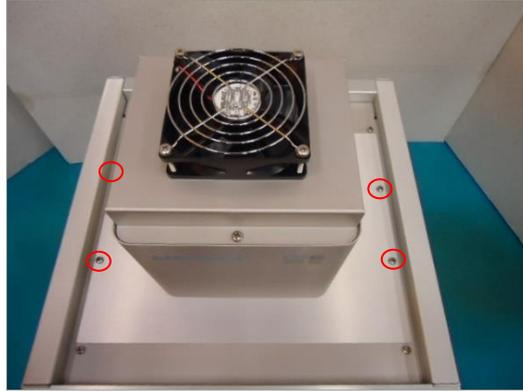
6. Center the Reflector Housing on the Light Shield. When the desired position is achieved, tighten the Securing Brackets to the Light Shield (Figure 8).
