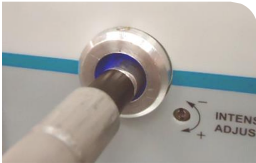
Figure 6. Insert Lightguide into Lightguide Mount
