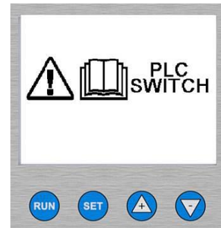
Figure 24. Message to Set PLC Switch
