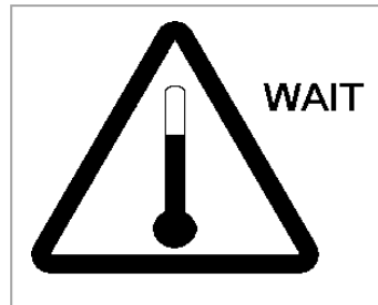
Figure 29. LED Head Has Overheated
