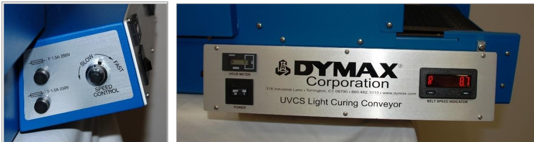
Figure 6. Conveyor Control Panel
