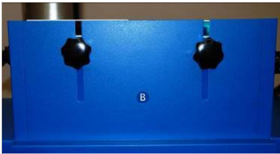
Figure 9. LED Array Height Adjustment
