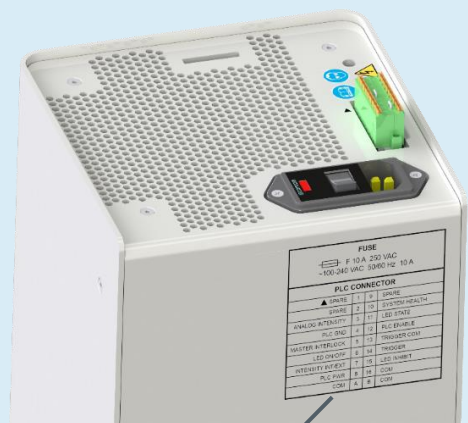
Figure 8. PLC Connector Pin Reference
