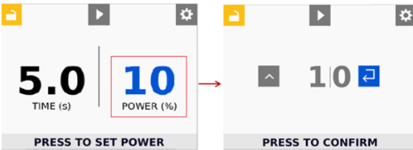
Figure 32. Power Level Screen
