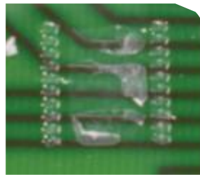
Figure 5. Day 3 at RT Adhesive under the component was soft with a wet surface.
