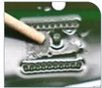
Figure 3. Day 1 at Room Temperature Adhesive under component was soft and had a wet surface
