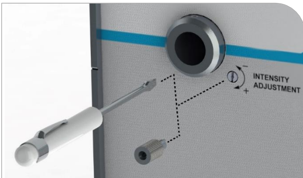
Figure 39. Adjust Intensity with a Tool or the Removable Knob
