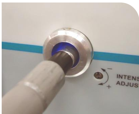
Figure 6. Insert Lightguide into Lightguide Mount
